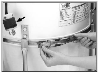
Figure 3. Unplug machine when emptying bags.
